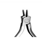
NANCE LOOP FORMING PLIER - Four steps (3, 4, 5 and 6mm) allow precision loop forming. Serrated beak on one side prevents wire slippage. Carefully beveled edges prevent wire scoring. Utility groove at the base of beak for closing formed loops. Wire up to .022".
